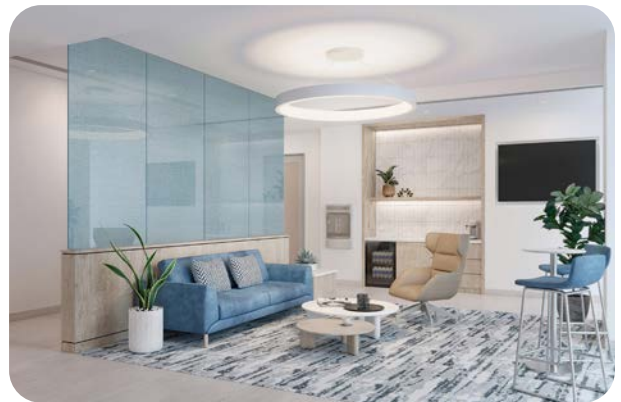
Laminated glass with blue fabric interlayer
