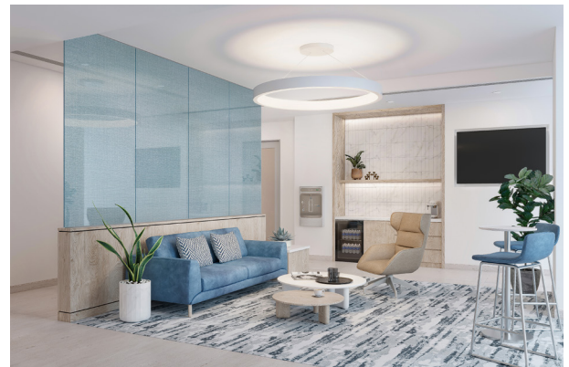
Laminated glass with blue fabric interlayer.
