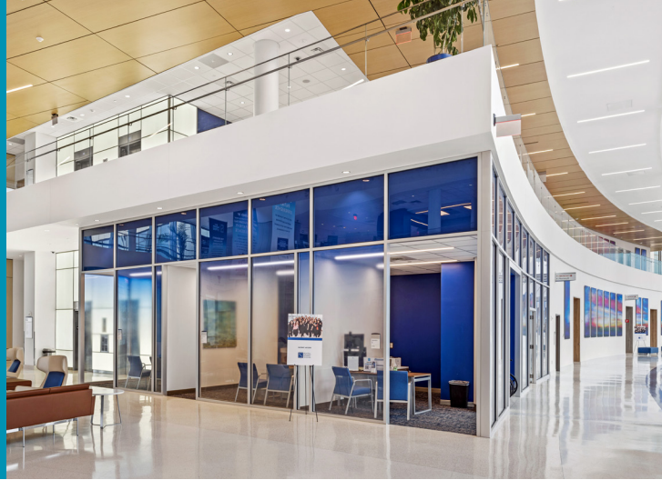
Laminated glass with printed gradient interlayer + backpainted glass above.
